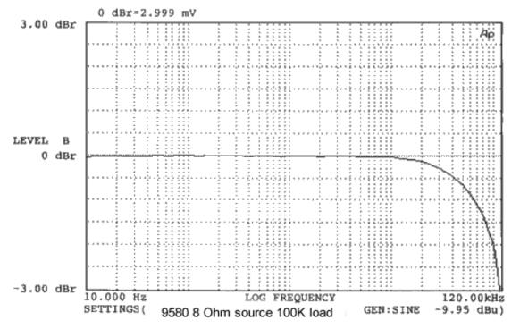
Typical response 8 Ohms source 100K Ohms load.
