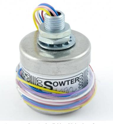
balanced or unbalanced. Centre tap on input for phantom powering etc. Available with leads or for PCB mounting. May also be used with primary and secondary reversed as a step-down transformer for use with a CD player or similar device. In this mode the transformer will isolate and balance the output as well as reducing the impedance and output level by 12 to 14 dB for driving a 600 ohm balanced line.
