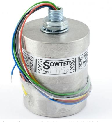
and phase balance over the full bandwidth. For cartridges in the range 3 to 15 ohms 5 Hz to 120 kHz. Configurable for 1:5 ratio by connecting the two secondary windings in parallel. DC resistance Primary: 0.45 Ohms. Secondary 66 Ohms. Two transformers are required for stereo. Mumetal can.
