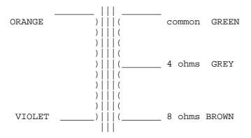
SA11 SE Output for 211 10000 ohms, 25 Watts at 20 Hz, 70 mA, 15 Hz to 70 kHz,
