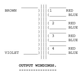
There are FOUR EQUAL SECONDARY WINDINGS which can be arranged for loads of 1, 4, 8/9 or 15/16 ohms thus:-
