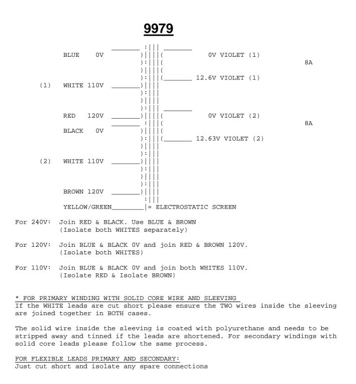
NOTE: A certain amount of mechanical hum is prevalent in mains transformers and can be amplified when bolting to your metal work. Therefore you may find a small rubber gasket or similar material is worth fitting to quieten this hum to its' minimum, but please ensure the frame is grounded to the supply safety earth.
