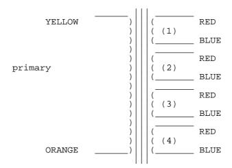
There are FOUR EQUAL SECONDARY WINDINGS which can be arranged for loads of 1, 4, 8/9 or 15/16 ohms thus:-
