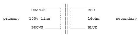
100v line transformer, speech quality, 30 watt output, into 16ohm load.
