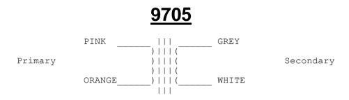
**9705** Single Ended triode to line output 4:110k/600 ohms single ended output transformer. 40 H primary. Up to 30 mA dc. Max output +24 dBu (12 volts). Total dc resistance ref secondary 96 ohms. Colour coded leads. Size D. M6 core
