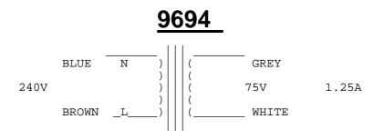
Mains earth can be connected to the fixing bolt thus earthing the core and end shields.
