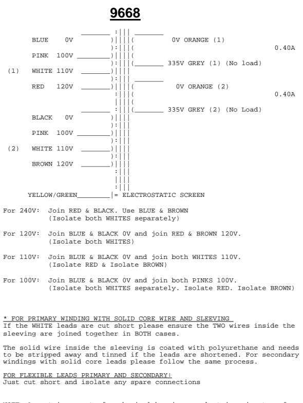
NOTE: A certain amount of mechanical hum is prevalent in mains transformers and can be amplified when bolting to your metal work. Therefore you may find a small rubber gasket or similar material is worth fitting to quieten this hum to its' minimum, but please ensure the frame is grounded to the supply safety earth.
