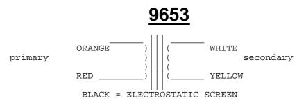
Cartridge transformer for High Impedance applications. Ratio 1:6, Cartridge Z nominal 8 ohms (4 - 16 ohms) Frequency response 20Hz -  $60 \, \mathrm{kHz}$ .
