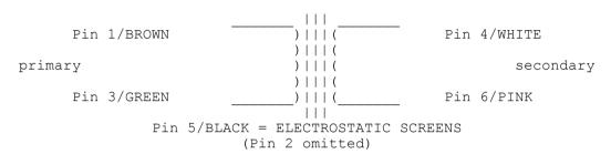
**9262** – replacement for 8230 Available on PCB pins (style "c") or colour coded leads (style "f")
