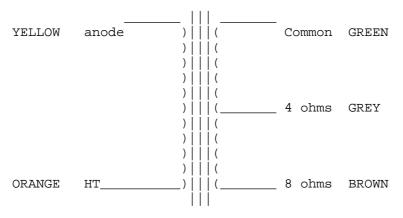
15 WATT SINGLE ENDED OUTPUT TRANSFORMER type number 9583 Primary impedance 2000 Ohms. Secondary impedance 8 Ohms. LF Cut off -3.0 Db at 20Hz. Source 400 Ohms DC current 100 mA. Fully shrouded upright type. Colour coded leads. Weight 4.2 Kg approx. Dimensions 117(above chassis) x 96 x 110 mm.
