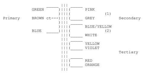
Join two secondaries in parallel for 10:1 ratio or in series for 5:1)
