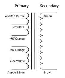
Further Information: 9511: 50W Push-Pull Output Transformer  $8\Omega$  secondary winding  $Z_{Pri} = 7k\Omega$ Screen Taps at 40%
