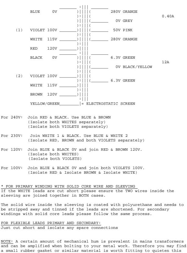
and can be amplified when boiling to your metal work. Therefore you may find a small rubber gasket or similar material is worth fitting to quieten this hum to its' minimum, but please ensure the frame is grounded to the supply safety earth.
