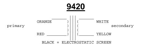
Cartridge transformer for High Impedance applications. Ratio 1:6, Cartridge Z nominal 40ohms (25 - 100 ohms) Frequency response 10Hz - 40kHz.
