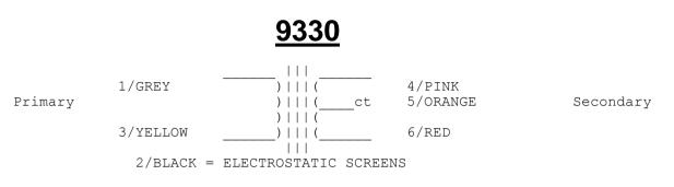
**9330 Pulteq EQP-1A 2k5/10KCT Amp input** Ratio 1:2 CT. Max input level +20 dBu. Sowter designed transformer similar to Triad HS-29. Internal electrostatic shield to ensure good common mode rejection for accurate phase splitting at high frequencies. Mumetal can with colour coded leads or PCB pins.
