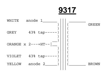
The transformer will need to be mounted at 90 degrees to the original to fit the space, and will need to be raised up to allow for the wires to fit onto the tag board in the same way as the old transformer
