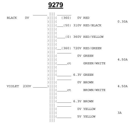
$\underline{\text{Note:}}$  A certain amount of mechanical hum is prevalent in mains transformers and can be amplified when bolting to your metal work. Therefore you may find a small rubber gasket or similar material is worth fitting to quieten this hum to its' minimum, but please ensure the frame is grounded to the supply safety earth.
