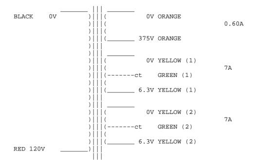
$\underline{\text{Note:}}$  A certain amount of mechanical hum is prevalent in mains transformers and can be amplified when bolting to your metal work. Therefore you may find a small rubber gasket or similar material is worth fitting to quieten this hum to its' minimum, but please ensure the frame is grounded to the supply safety earth.
