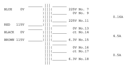
$\underline{\text{Note:}}$  A certain amount of mechanical hum is prevalent in mains transformers and can be amplified when bolting to your metal work. Therefore you may find a small rubber gasket or similar material is worth fitting to quieten this hum to its' minimum, but please ensure the frame is grounded to the supply safety earth.
