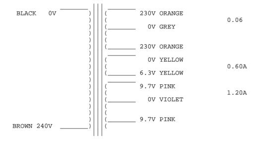
Note: A certain amount of mechanical hum is prevalent in mains transformers and can be amplified when bolting to your metal work. Therefore you may find a small rubber gasket or similar material is worth fitting to quieten this hum to its' minimum, but please ensure the frame is grounded to the supply safety earth.
