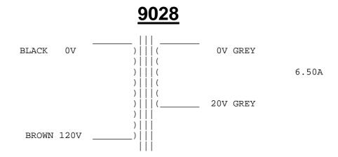
If the Grey leads are cut short please ensure the TWO wires inside the sleeving are joined together in BOTH cases.
