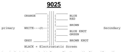
In series for 2.4k ohms i.e: join Brown + Blue Knot. Use Blue and Brown Knot
