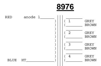
There are FOUR EQUAL SECONDARY WINDINGS which can be arranged for loads of 300, 150, 75 or 18 ohms thus:-
