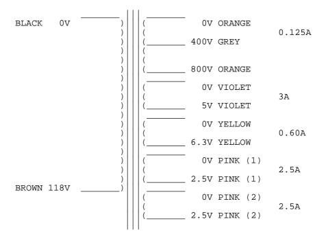
Note: A certain amount of mechanical hum is prevalent in mains transformers and can be amplified when bolting to your metal work. Therefore you may find a small rubber gasket or similar material is worth fitting to quieten this hum to its' minimum, but please ensure the frame is grounded to the supply safety earth.
