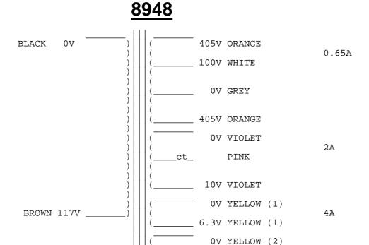
Note: A certain amount of mechanical hum is prevalent in mains transformers and can be amplified when bolting to your metal work. Therefore you may find a small rubber gasket or similar material is worth fitting to quieten this hum to its' minimum, but please ensure the frame is grounded to the supply safety earth.
