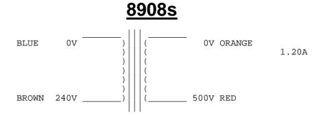
$\underline{\text{Note:}}$  A certain amount of mechanical hum is prevalent in mains transformers and can be amplified when bolting to your metal work. Therefore you may find a small rubber gasket or similar material is worth fitting to quieten this hum to its' minimum, but please ensure the frame is grounded to the supply safety earth.
