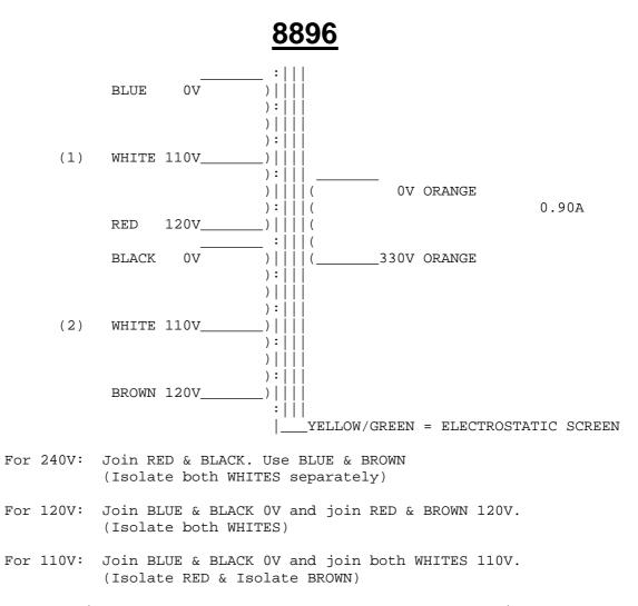
If the White leads are cut short please ensure the TWO wires inside the sleeving are joined together in BOTH cases.
