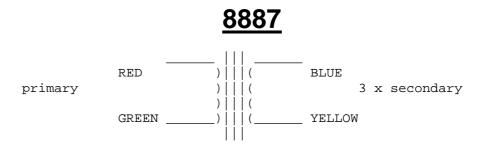
600ohm / 3x 600ohm for line splitter use
