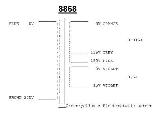
Note: A certain amount of mechanical hum is prevalent in mains transformers and can be amplified when bolting to your metal work. Therefore you may find a small rubber casket or similar material is worth fitting to quieten this hum to its' minimum, but please ensure the frame is grounded to the supply safety earth.
