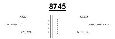
Primary impedance 3500ohm, (source 3000ohm) Secondary impedance 3500ohm LF cutoff -0.5dB at 20Hz, dc. current 7mA
