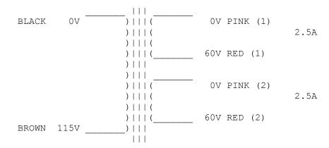
Note: A certain amount of mechanical hum is prevalent in mains transformers and can be amplified when bolting to your metal work. Therefore you may find a small rubber casket or similar material is worth fitting to quieten this hum to its' minimum, but please ensure the frame is grounded to the supply safety earth.
