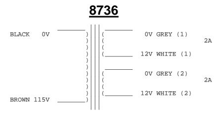
$\underline{\text{Note:}}$  A certain amount of mechanical hum is prevalent in mains transformers and can be amplified when bolting to your metal work. Therefore you may find a small rubber casket or similar material is worth fitting to quieten this hum to its' minimum, but please ensure the frame is grounded to the supply safety earth.
