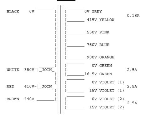
You will note that the Primary is built up in sections and the two wires in the White and Red sleeves must always be individually joined to make the primary circuit complete. Spare connections not required can be cut short, each colour joined separately and isolated. The solid wire inside the sleeving is coated with polyurethane and needs to be stripped away and tinned if the leads are shortened.
