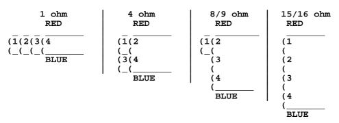
8624 10watt push pull output transformer Primary Ra-a 9Kohm, 230mA dc per side Secondary for load of 1,4,8 & 16 ohm.
