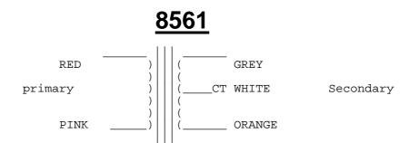
200 ohms 1:1ct Frequency Response 40Hz - 15kHz Mic levels.
