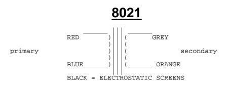
25 ohm/ 25 ohm 2.5 watts Turns ratio 1:1
