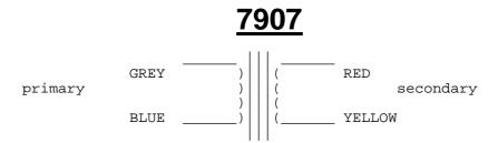
300 watt output transformer Primary - 4ohm Secondary - 100v line Frequency response 30Hz - 12kHz (3dB point)
