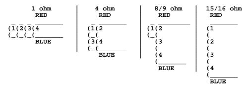
6000 ohm Ra-a , dc current = 80mA per side Secondary for 1,4.8 or 16 ohms 40watts output.
