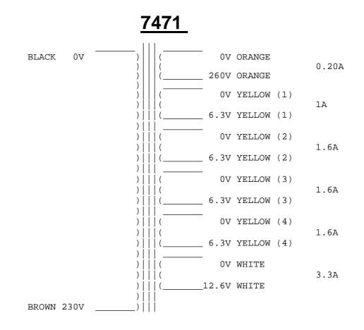
\* FOR PRIMARY WINDING WITH SOLID CORE WIRE AND SLEEVING The solid wire inside the sleeving is coated with polyurethane and needs to be stripped away and tinned if the leads are shortened. For secondary windings with solid core leads please follow the same process.
