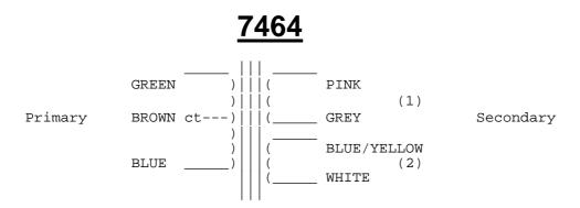
Join two secondaries in parallel for 10:1 ratio or in series for 5:1
