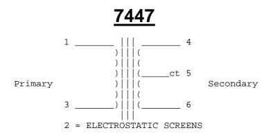
Primary 600 ohms / secondary 150 ohms ct Turns ratio 2:1 step-down
