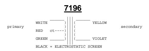
200 ohms Primary - Turns Ratio 1:3.16 Max input level 1.5V at 30Hz With electrostatic and electromagnetic screening.
