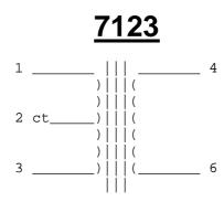
600ohm/600ohm balancing transformer. Turns ratio 1:1 Maximum Level +12db at 30Hz, Frequency response +/- 1db 20Hz - 20kHz. Electrostatic screen . Pins for direct soldering to pcb.
