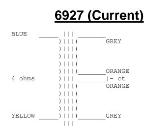
Sowter transformer type 6927 is an output transformer for use with electrostatic loudspeakers. For 4 ohms Primary at 20 volts, i.e:100 watts. Secondary is 2000V centre tapped
