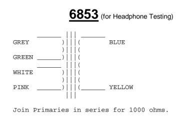
Primary Z = 1000 ohms Secondary Z = 8 ohms Turns Ratio = 10.7:1 step-down Frequency Range = 250Hz-4.5kz
