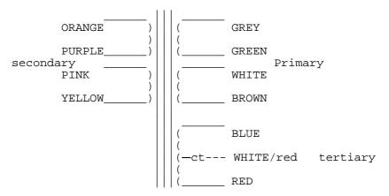
Pri 12.5kohm in two halves sec 600 ohm in two halves and 24 ohm tertiary winding max level +24dB at 20Hz
